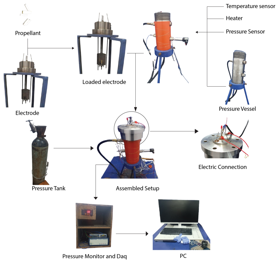
Figure 3.3: Working of Crawford Bomb Setup.
